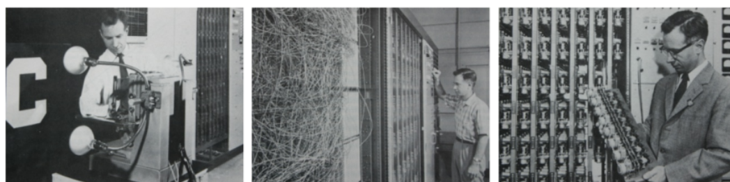
Figure 1.14 Illustration of the Mark 1 perceptron hardware. The photograph on the left shows how the inputs were obtained using a simple camera system in which an input scene, in this case a printed character, was illuminated by powerful lights, and an image focused onto a 20 \times 20 array of cadmium sulphide photocells, giving a primitive 400-pixel image. The perceptron also had a patch board, shown in the middle photograph, which allowed different configurations of input features to be tried. Often these were wired up at random to demonstrate the ability of the perceptron to learn without the need for precise wiring, in contrast to a modern digital computer. The photograph on the right shows one of the racks of learnable weights. Each weight was implemented using a rotary variable resistor, also called a potentiometer, driven by an electric motor thereby allowing the value of the weight to be adjusted automatically by the learning algorithm.
